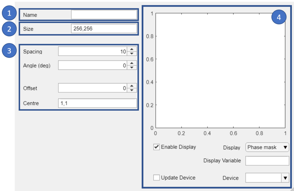
Fig. 4.27: Overview of ui.simple.linear graphical user interface. The layout consists of: (1) Output variable name; (2) Size of pattern (mostly used on ui.simple.* GUIs); (3) Controls for the method; and (4) Pattern preview window.
